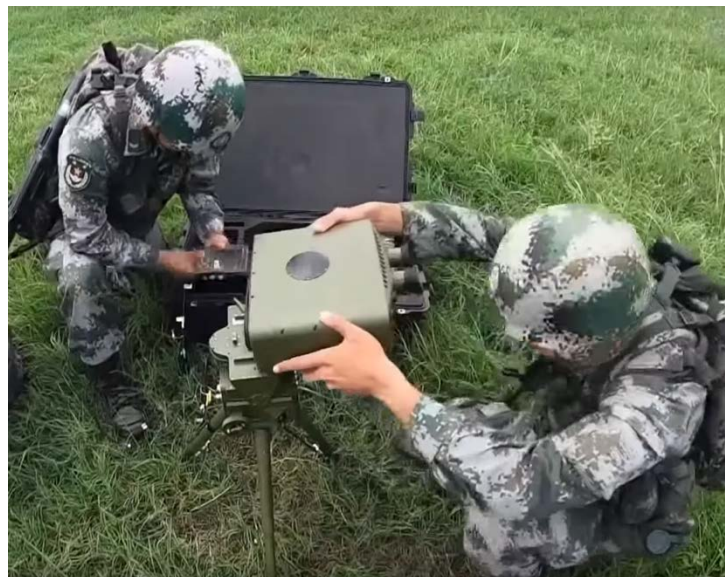
Figure 2: Soldiers of the 83rd Air Assault Brigade set up a laser designator.
